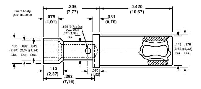
Min hole depth (socket) .375 (9,53)
